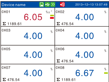
Digital display Measured values, channel number, engineering unit, alarm status and accumulative message,all of them will be displayed in digital form.
