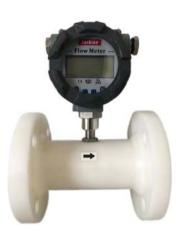
This kind of measured liquid has no impurities such as fiber and particles. The movement viscosity is lower than 5×10-6m2/s at working temperature. If the viscosity is higher than 5×10-6m2/s, the flow meter should be calibrated in the liquid before use. It can finish batch control, alarm and etc, if matched with special digital controllers. It is also the ideal meter for flow measuring and energy saves.
