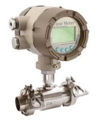
and energy saves. Hygienic Turbine Flow meters provide a durable and cost efficient ways to measure the liquid fluids in excellent precise and stable repeatability. This sanitary TUF is designed for the dairy, beverage, food processing and pharmaceutical industries. Such as for clean water, milk, palm oil, edible oil, vegetable oil, fish oil flow measurement and so on. The design of this type flowmeter is also suitable for cleaning-in-place (CIP).
